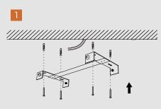
Fix light bracket with screw and plastic anchor into the ceiling,make sure the bracket is firmly installed
