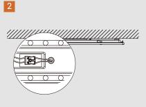
Connect the L、N wires to the terminal
