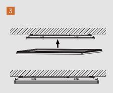
Install the lampshade, screw the latch to secure the lampshade
