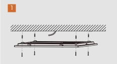
Fix light bracket with screw and plastic anchor into the ceiling,make sure the bracket is firmly installed
